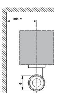
X/Y: Minimum distance with respect to the valve centre.
